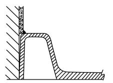
To prevent the possibility of water damage check all connections are water tight and that the tray is adequately sealed along the tiling line
