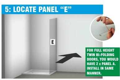
Slide **"PANEL E"** into the wall compensator. An optional self adhesive protective strip is supplied for applying to the bottom edge of the glass panels, see inset above. We **recommend** using this on a tiled floor setting.
