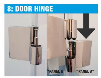
The hinge attached to **"PANEL A"** will have a spigot ready to accept **"PANEL D"**, above left. Ensure the spigot part of the hinge is on the outer side of the door, with the receiving pin pointing upwards, to ensure the rise & fall hinges open outward.
