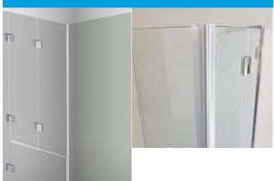
With the doors assembled and in the closed position, **ENSURE** that the magnetic profiles where the door(s) / fixed panels meet at the corner are parallel and the magnetic profiles come together for the full height of the doors.
