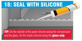
Silicone joint between floor / shower tray both "PANEL A / E". Allow suitable cure time for silicone (this may be 24 hours depending on the variety use). FOLLOW THE MANUFACTURERS GUIDELINES WHEN USING SILICONE SEALANT.
