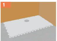
Locate ShowerDec® in the corner to which it is going to be finally positioned & mark lines around the outer edge.
