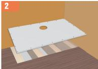
Remove the floor within the marked area to a depth of 18mm to accept ShowerDec®.
