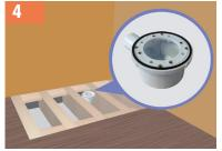
Connect the trap body to your outlet pipework, position between joists and centrally beneath the hole in the ShowerDec®.
