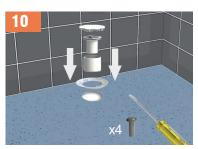
Once the floor covering is laid, screw into position the trap clamping ring using the bolts provided, ensuring the inner cup & dip tube can still be removed.
