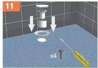
Once the floor coving is laid, screw into position the traps clamping ring using the bolts provided ensuring the inner cup and dip tube can still be
