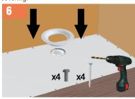
Attach flange to the trap body using the 4 bolts provided, ensuring that the rubber seal is in place. Secure flange to ShowerDec®, there are 4 countersunk indentations in the flange to assist with this.
