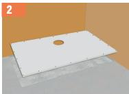
Excavate the floor within the marked area to a sufficient depth of 24mm to accept ShowerDec®.
