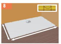
Ensure that the ShowerDec® is well supported and completely level.
