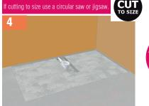
Remove ShowerDec®. Decide upon the position of the waste pipe knocking out a hole in the adjacent wall if required. It will be necessary to remove an area to sufficient depth under the outlet position to accomodate the shower trap. (Approximate trap depth 95mm x 110mm wide).
